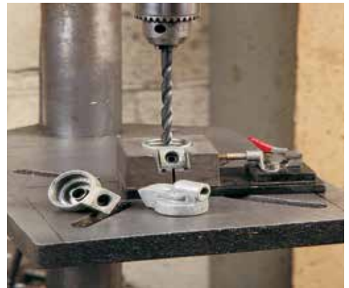
Plastic Steel Liquid offers a fast and economical way of making holding fixtures.
