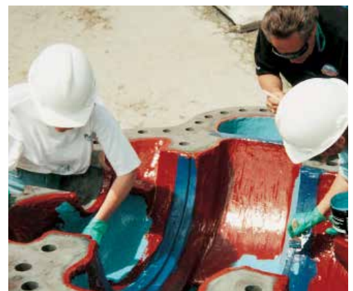
Brushable Ceramic provides pumps and other equipment with a smooth protective barrier against wear, abrasion, corrosion, erosion and chemical attack and it fills holes and voids in castings.
