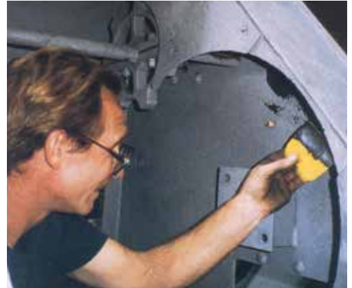
Plastic Steel, the first fortified epoxy repair compound is still one of the most effective for a wide range of general metal repair and rebuilding applications.
