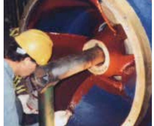
Ceramic Repair Putty protects equipment surfaces from damage due to wear and abrasion, extending service life and often eliminating the cost of replacement.
