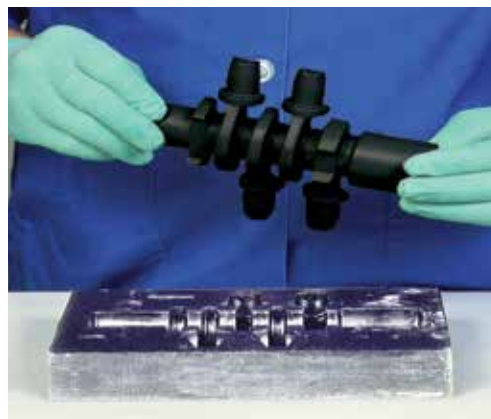
Use Flexane Liquids to mould small quantities of rubber parts easily and economically.
