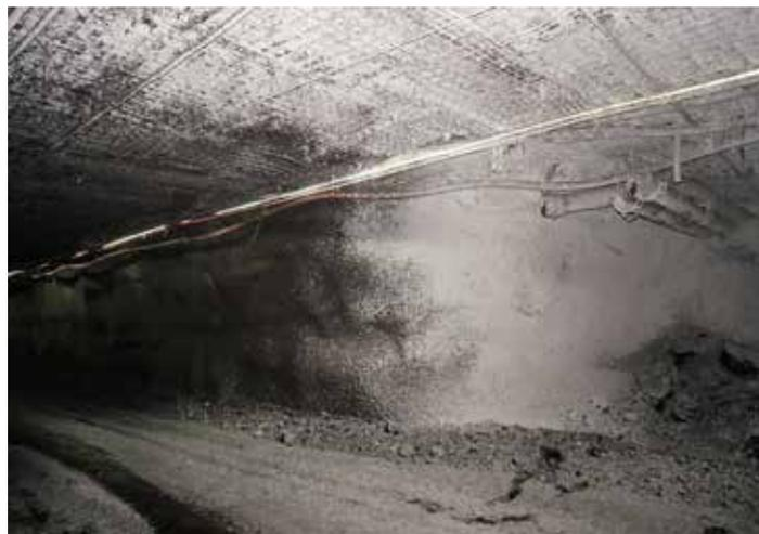
*Airo-Duster underground where Airo-Dust has been sprayed*
