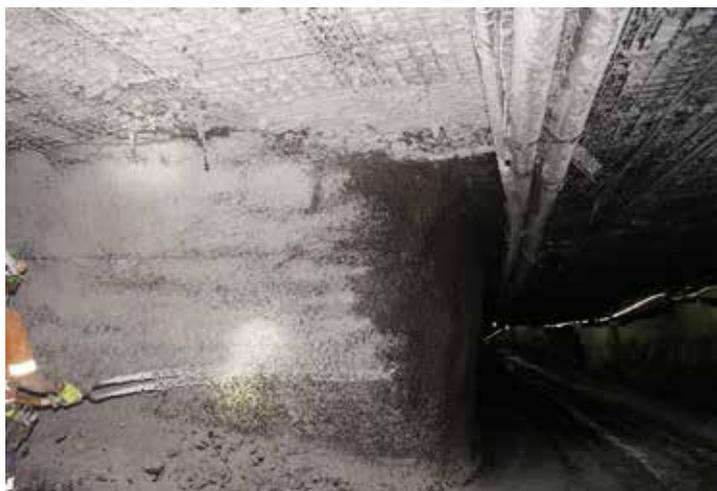
*RHS showing sprayed area with Airo-Dust and LHS not sprayed*
