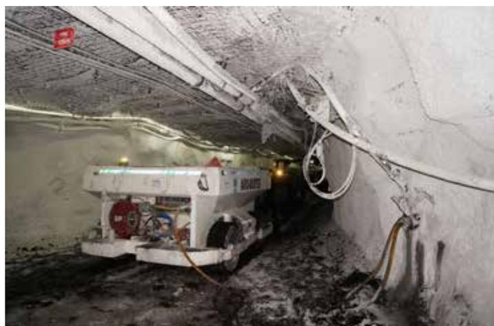
*Airo-Duster underground where Airo-Dust has been sprayed*
